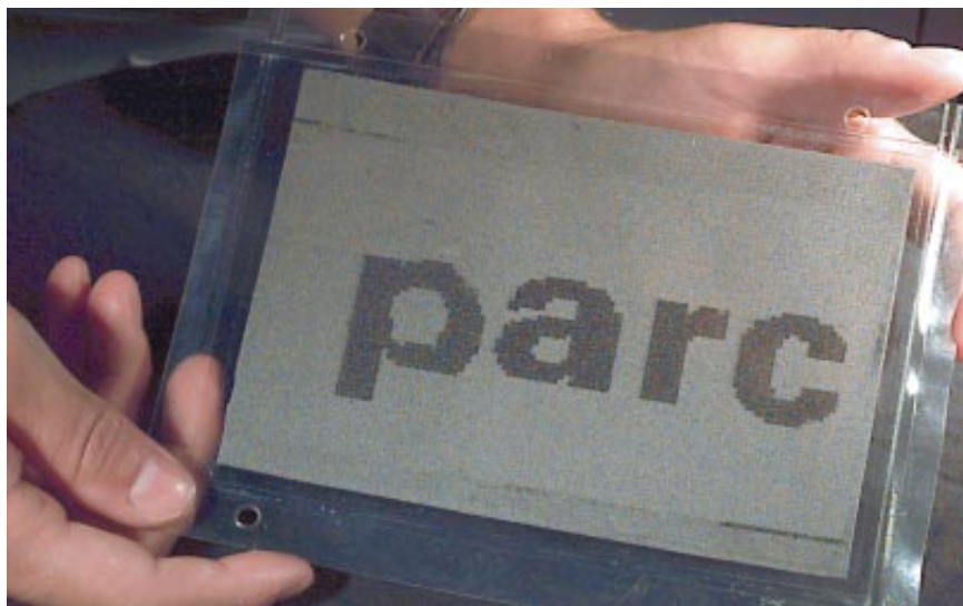
PROTOTYPE OF XEROX'S GYRICON DISPLAY, as thin as seven sheets of paper, will hold its image for months without power.
